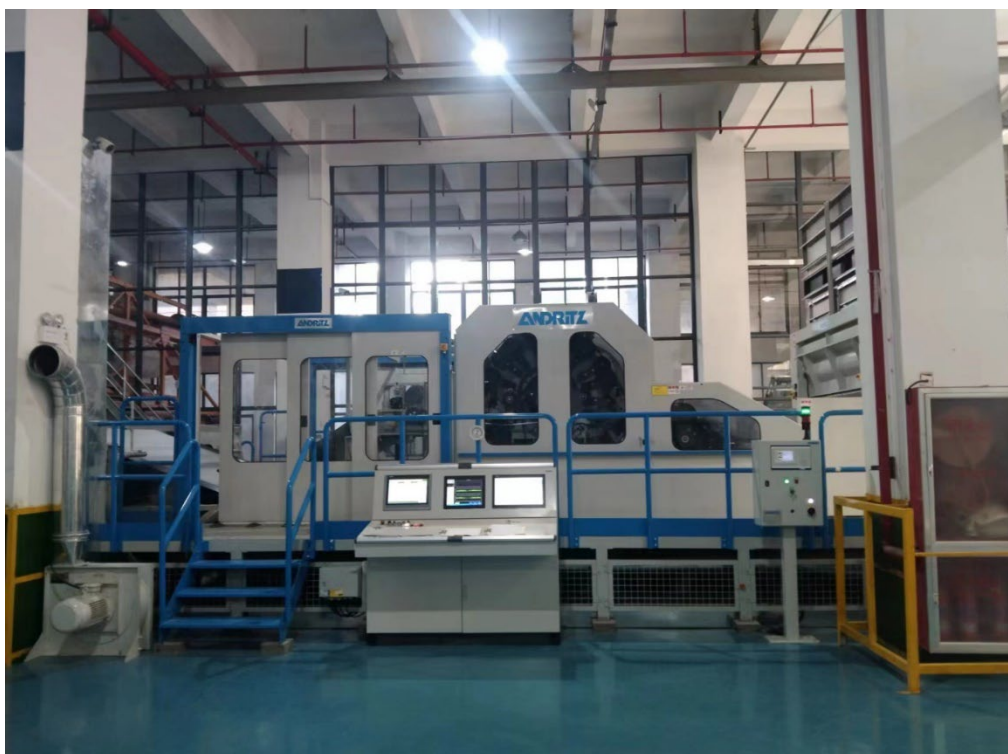
Third ANDRITZ needlepunch line in operation at Meisheng plant
